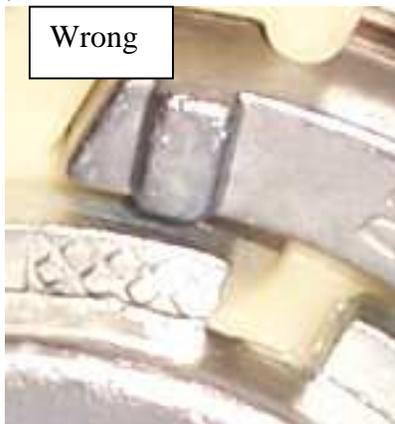
**The above picture is also NOT ACCEPTABLE.** You must readjust tensioner and rotate engine **clockwise** two times to TDC and re-check again before continuing with installation procedure. **Do not set pointer in crosshatch section.**
