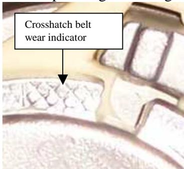
This picture shows the crosshatch belt wear indicator which is only on the new part.
