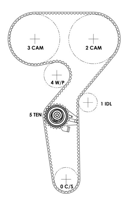
0: Crankshaft 1: Idler 2: CAM 3: CAM 4: WATER PUMP 5: Tensioner
