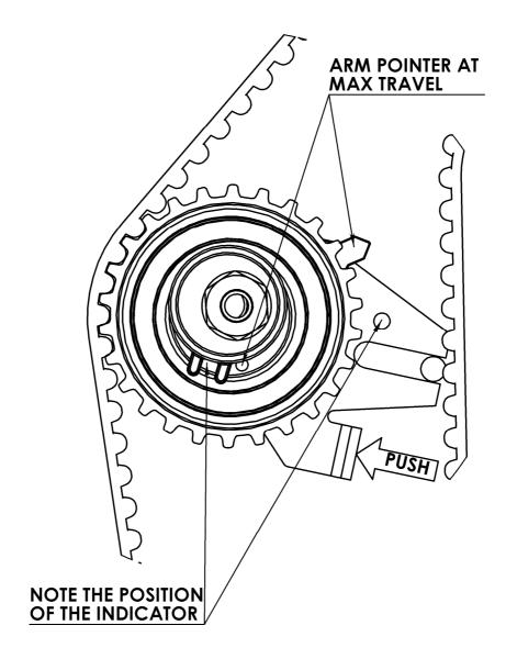
Figure 3: Proper Initial Setup of Tensioner
