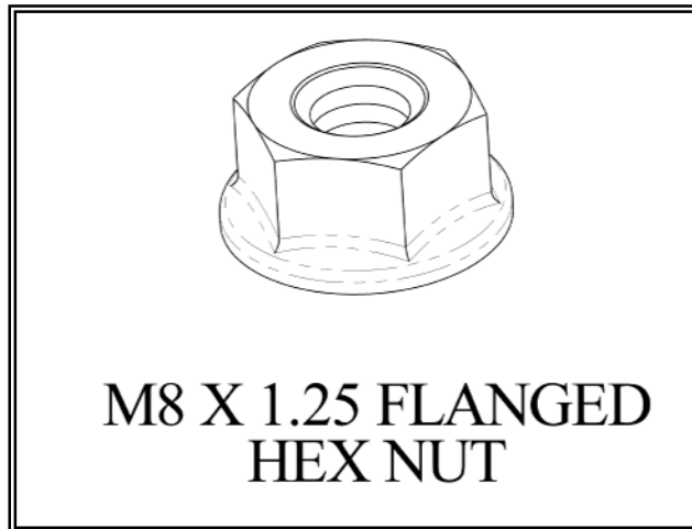
Figure 2: Flanged Hex Nut used for mounting the tensioner on the engine.
