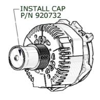
Step 5. Installation of the Cap:
