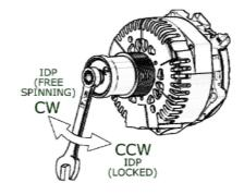
Step 4. Verification of the proper installation:
